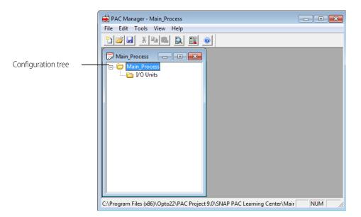
You can expand and collapse the folders to see or hide the I/O units and points in them. Closing the configuration tree is the same as closing the configuration file.
