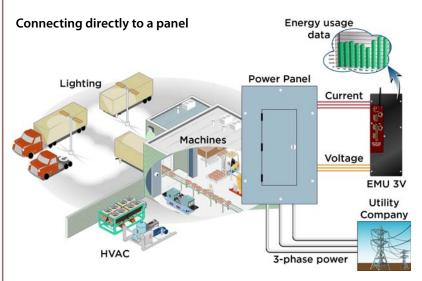
A total of 64 Modbus data items (over Ethernet and serial) can be monitored.
