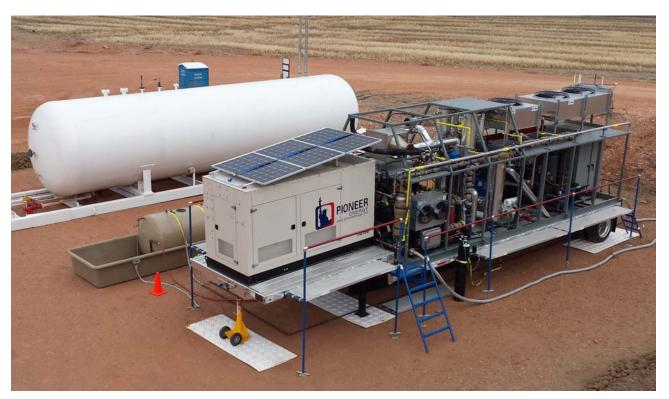
Pioneer Energy's MAGS system is shown here deployed at a well site in North Dakota. Processed gas is stored in the large tank.
