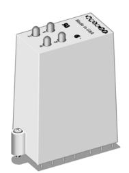
DC output modules are used for controlling or switching DC loads. Each module provides up to 4,000 Vrms of optical isolation between the field devices and the control logic.
