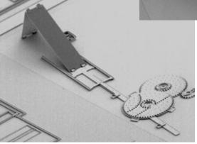
Two views of a tiny MEMS (Micro Electromechanical Systems) mirror. The mirror is approximately 100 micrometers wide, or about the diameter of a human hair.
