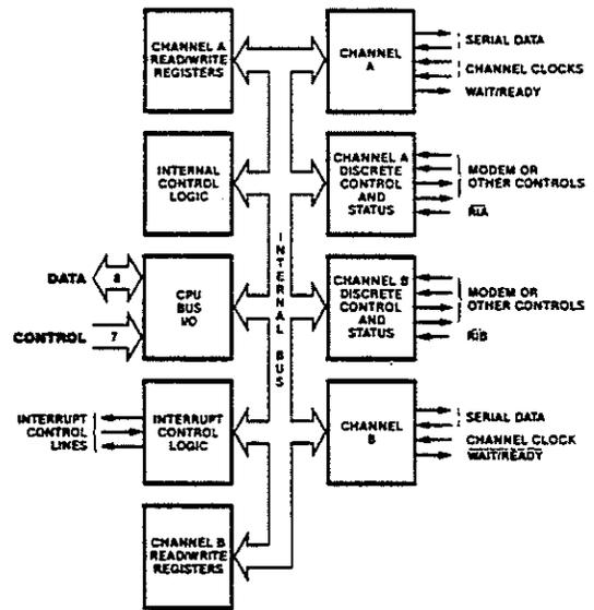
Figure 3. Block Diagram
