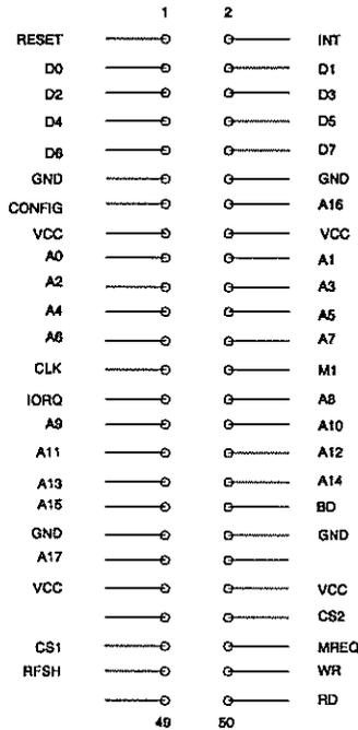
Figure 7 - Option Port Pinout
