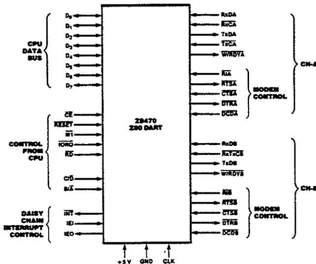
Figure 1. Pin Functions
