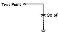
FIGURE 5 — NMOS EQUIVALENT TEST LOAD
