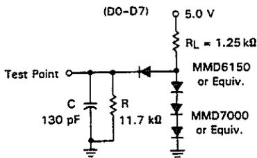
FIGURE 3 — TTL EQUIVALENT TEST LOAD
