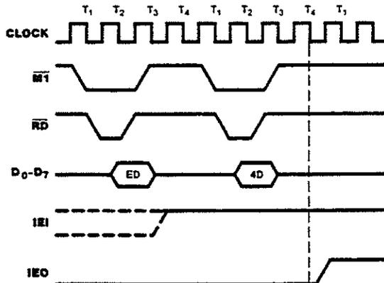
Figure 8. Return from Interrupt Cycle
