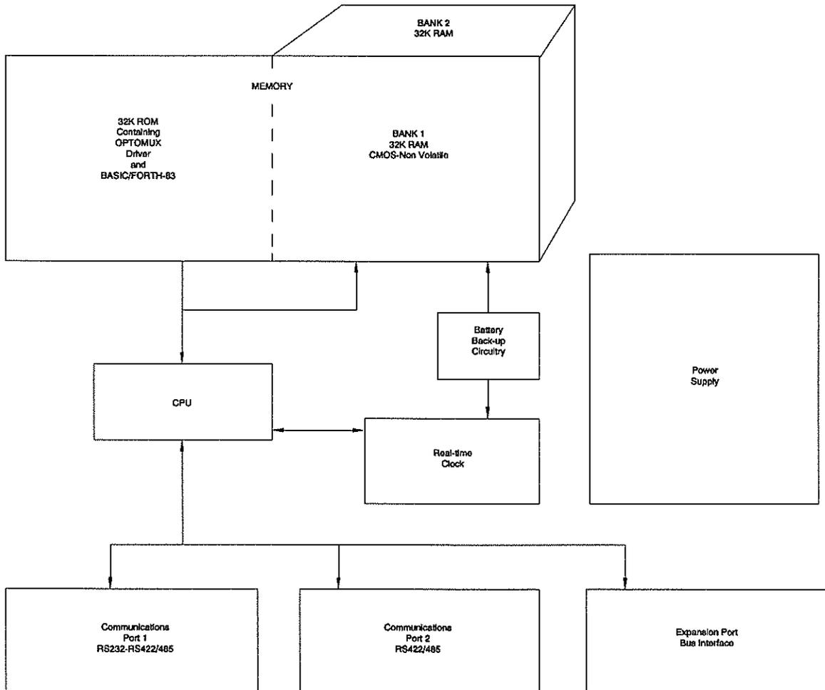
Figure 1 - LC4 Block Diagram
