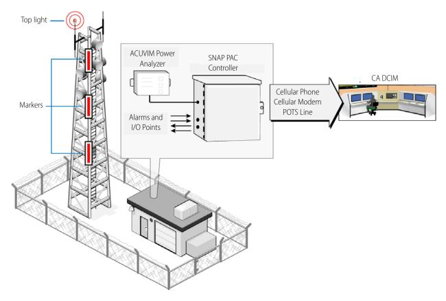
CANTV, the national telephone company of Venezuela, installed a packaged solution using Opto 22's SNAP PAC system to monitor and manage hundreds of remote telecom sites.
