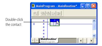
**4.** Assign the normally open contact to the Limit Switch by selecting bit 0 of the SNAP\_IRIO:I.Data[0] DINT.
