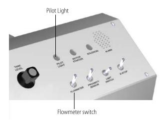
In this part of lesson 2, you've seen how you can configure and execute a watchdog. **15.** While the Ethernet cable is still unplugged, toggle the Flowmeter switch several times. **16.** Re-insert the cable, wait for communications to be re-established, and then notice that the flowmeter counts have increased.
