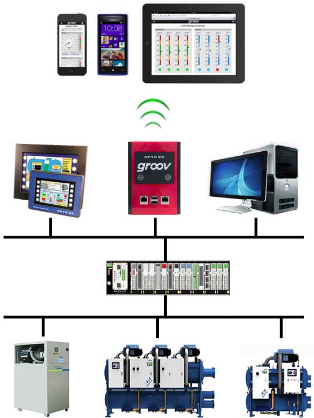
The BSE Energy Loop® Group Control System incorporates maglev chillers, cooling pumps, condenser pumps, and cooling towers in an automated and energy-saving central control system.
