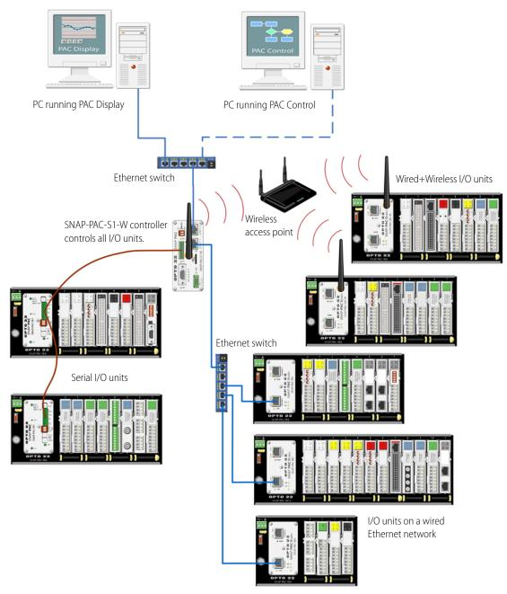
The Wired+Wireless SNAP PAC S-series controller is controlling three groups of I/O units: one group through its serial port, another through a standard 10/100 Mbps interface, and the third over a wireless LAN.
