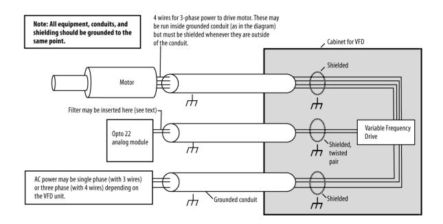
**TIP:** Do not run the power and control wires in parallel. If they are run in parallel (especially when close to each other), the harmonic noise from one wire is coupled to the other wire. Keep the power and control wires as far apart as possible. When they must cross, cross the power and control wires at 90-degree angles to prevent noise from being coupled to the control wires.
