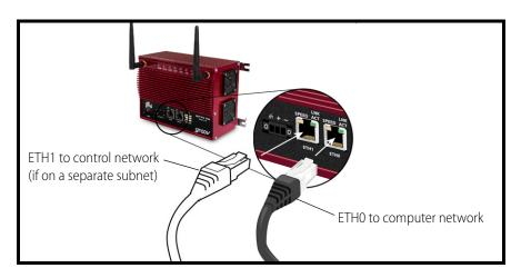
a. Connect an Ethernet cable from ETH0 to your computer's network.
